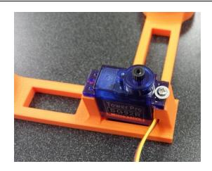
Use only one large screw to attach the servo from the bottom of the Rotator as shown.
