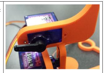
Using another large screw, attach the Rotator to the base servo as shown.
