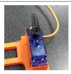
Place the servo horn onto the Rotator servo and gently\_rotate the horn clockwise as far as it will go. Remove the horn if necessary and replace it as shown.
