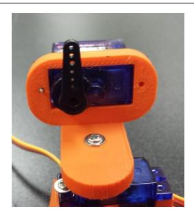
Attach the Large Gripper assembly to the Rotator servo with a large screw as shown.
