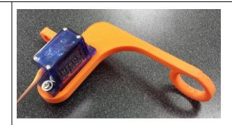
Place the servo horn onto the Base servo. **GENTLY** rotate the horn counterclockwise as far as it will go. The geartrain is soft nylon and will strip easily. Remove the horn and replace it as shown.
